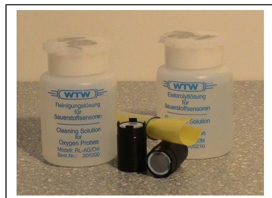
Cleaning solution for regeneration, Cathode cleaner, electrolyte solution, new membrane
