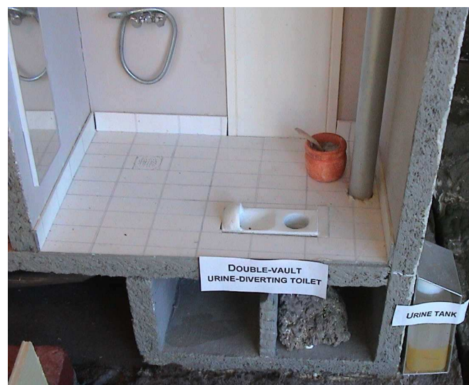
Figure 16: Squatting pan urine diverting toilet with double-vault from China
