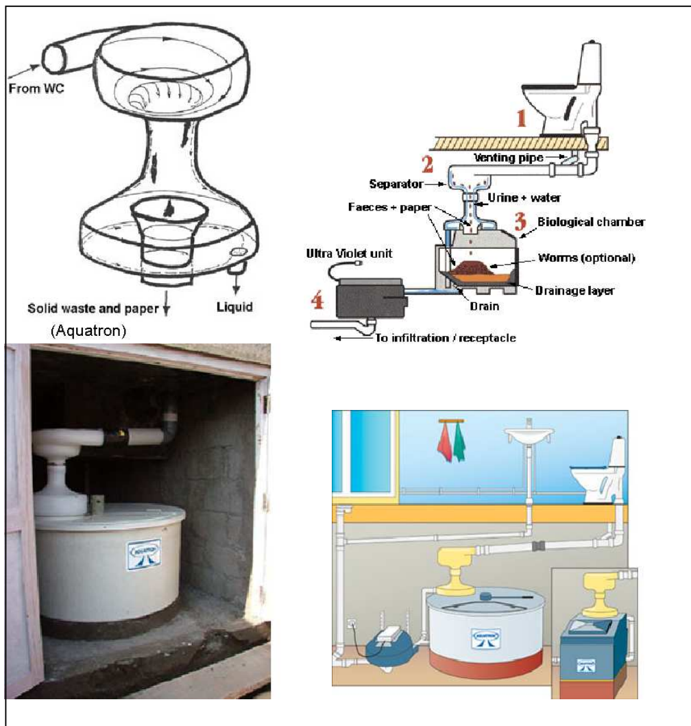
Figure 24: The whirlpool, surface tension separator Aquatron and its function where the faecal water (FW) is separated into liquids and solids (Vinnerås, 2002, http://www.aquatron.se )
