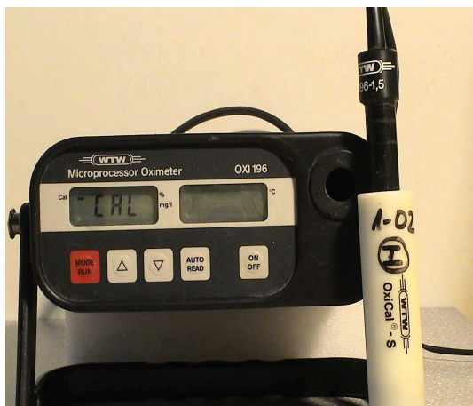
Figure 5: Oximeter with an electrode in the calibration vessel
