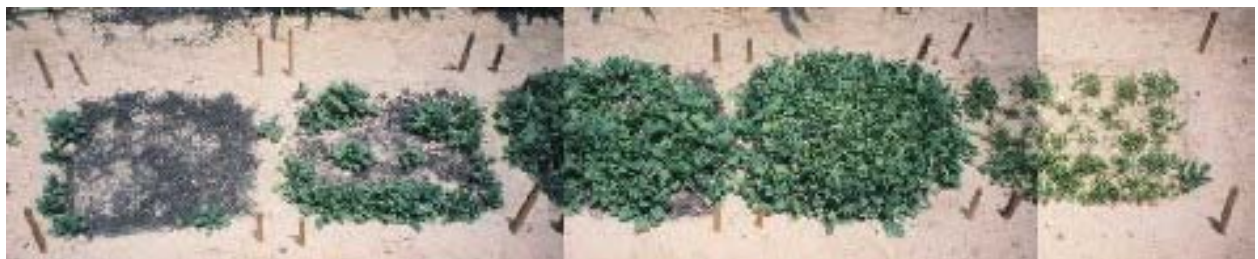
Photo 18: Development of Garghir (from left to right: Sand with 30 l dried sludge, Sand with 10 l dried sludge, Sand with 30 l converted sludge, Sand with 10 l converted sludge, Sand without additions)
