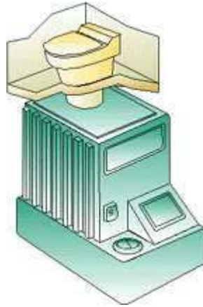
Figure 17 : Clivus Multrum composting toilet (Source: Clivus Multrum)
