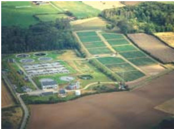
Fig. 4: KOLDING SLUDGE REED BED SYSTEM (DENMARK)
