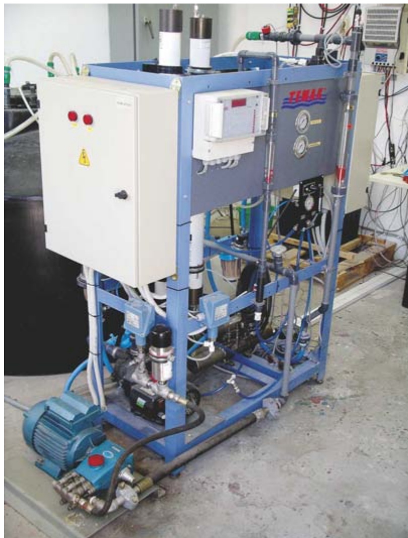
Fig. 1: SMALL REVERSE OSMOSIS DESALINATION UNIT 2.2 m 3 /DAY
