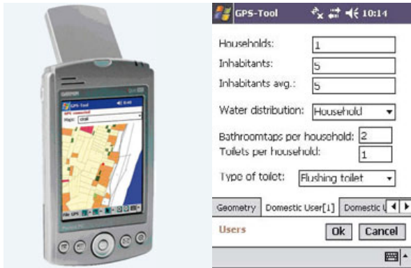
Fig. 2: THE GPS-BASED DATA ACQUISITION TOOL ADAPTED TO THE NEEDS OF THE DSS; THE COLLECTION OF INFORMATION REQUIRED FOR THE DESIGN AND COMPARISON OF POSSIBLE SOLUTIONS IS ENSURED.
