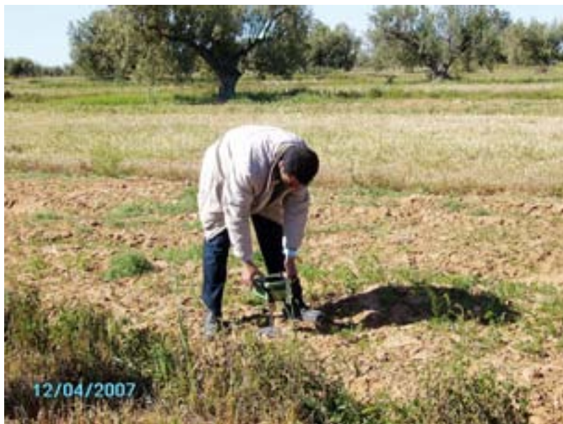
▲ Fig. 3: MEASUREMENT OF SOIL COMPACTION WITH A PENETRO METER
