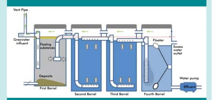
The system is airtight and watertight. Grey arrows indicate the flow direction of GW in the 4 barrels and the green arrows indicate the flow direction of gases that are produced during the digestion process, which are vented through a pipe above the roof level of the house. No odor is detected at the site.
