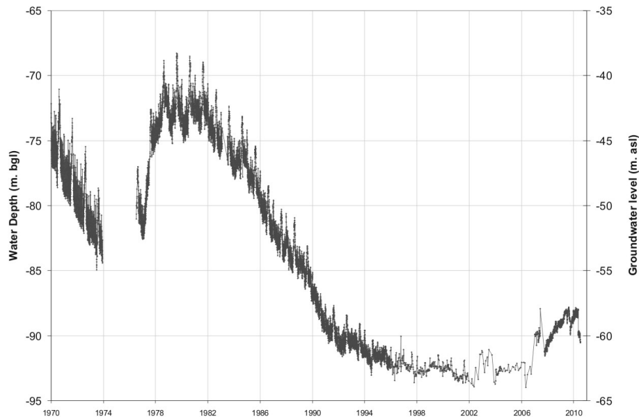
Figure 1: Piezometrical level (m) in a monitored borehole in Bondues (Fr), from 1970 to 2010.
