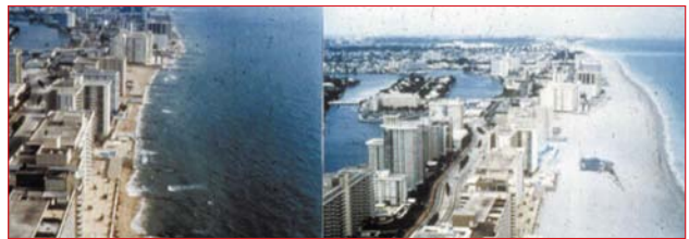
Before and after: beach nourishment along Miami coastline.
