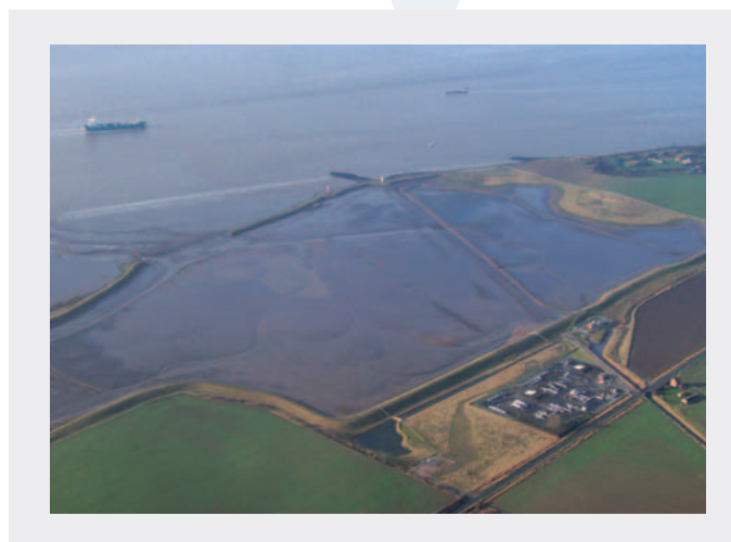
Figure 16. Example of habitat creation through managed realignment at Paull Holme Strays, Humber estuary. Credit: IECS, University of Hull.
